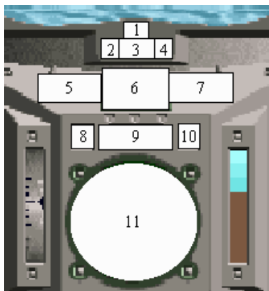
Figure 9 Detailed view of the periscope, rudder, and sonar controls: (1) periscope stop button, (2) periscope left button, (3) periscope angle, (4) periscope right button, (5) rudder left button, (6) rudder dial, (7) rudder right button, (8) active sonar light, (9) sonar switch, (10) passive sonar light, (11) sonar screen.
