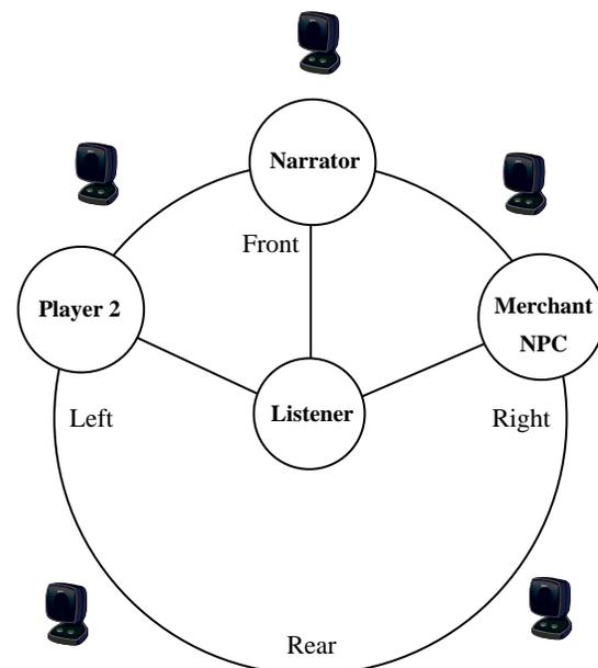
Figure 3. Sound Stage with 5-speaker surround sound configuration shown.
